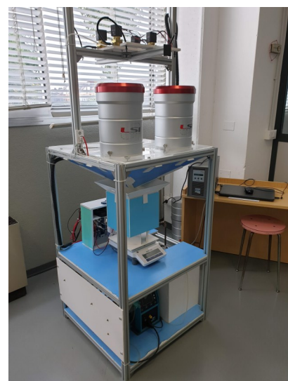
▶ Calibration apparatus designed and built by the WMO-CIMO Lead Center on Precipitation Intensity - Benedetto Castelli
